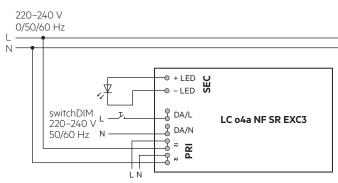
Device with loop through wiring function.
